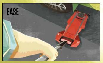
Their contoured, low-profile lift arm easily fits under vehicles and can be lifted higher than the competition. Crowned wheels allow for easier maneuvering, while a front wheel yoke, arm grease fittings and advanced retention system are stronger and easier to maintain.
